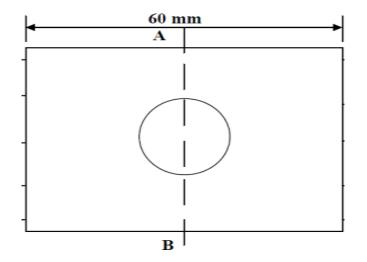
**AIM:** To perform a stress analysis of a rectangular plate with circular hole using analysis software ANSYS.
