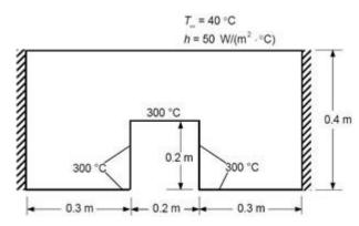
10. Solve the 2-D heat conduction problem for the temperature distribution within the rectangular plate. Thermal conductivity of the plate, KXX=510 W/(m-K).
